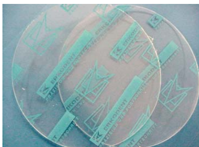
Figure 7. The blanks (foils) have a separating layer. Make sure this is used model side down.
