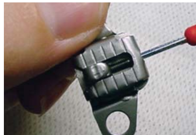
Figure 25. Insert the key to the screw and wind the hook to the middle position.
