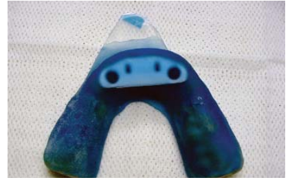
Figure 31. Embedded platform the acrylic was cured under pressure.
